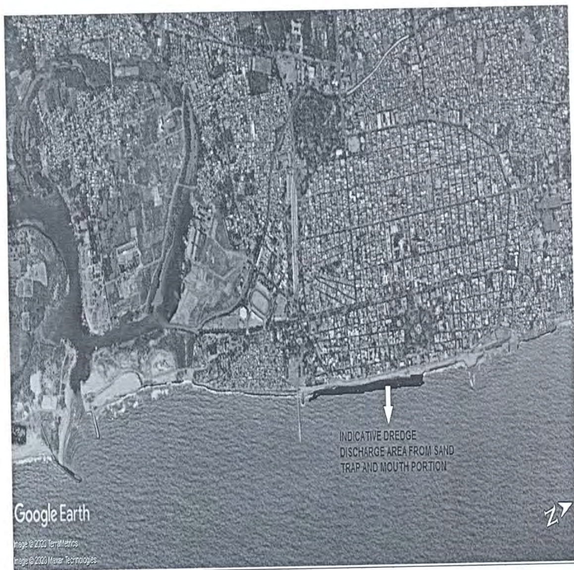
FIG 4.0 DREDGE DISCHARGE AREA FOR MAINTENANCE DREDGING AT MOUTH PORTION, ENTRANCE CHANNEL AND SAND TRAP AREA
